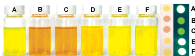
Figure 1. (Left) Color changes of solutions of 1 and various analytes. A, no analyte; B, L-cysteine; C, L-homocysteine; D, bovine serum albumin; E, L-glycine; and F, n -propylamine. (Right) Co-spots of 1 ( 1.0 \times 10^{-3} M) with and without various analytes ( 1.0 \times 10^{-3} M) under visible and UV light.
